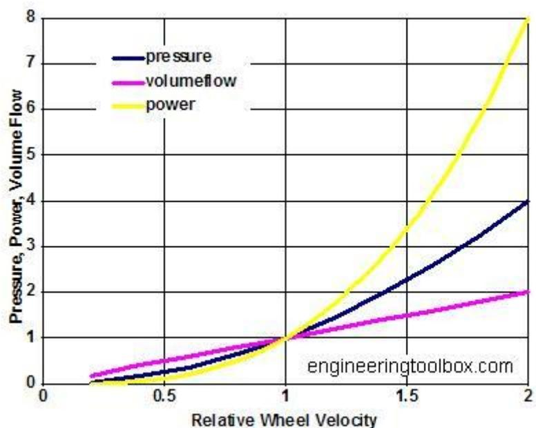
*Variable frequency drives permit users to consume the least amount of power to obtain desired pressure and flow*
