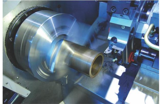
*Lathe – Low precision CNC machines like this lathe can often be completely controlled by a smart inverter, providing a low cost solution with all required features and functionality.*
