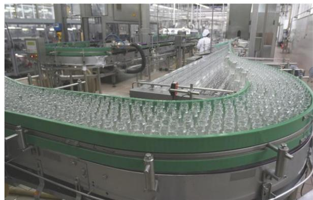
*Conveying system – A smart inverter can provide local control of a conveying line, allowing an operator to make speed adjustments as required.*
