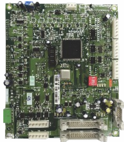
System Control Board of an i4 Series UPS - The DSP based digital control advantage!
